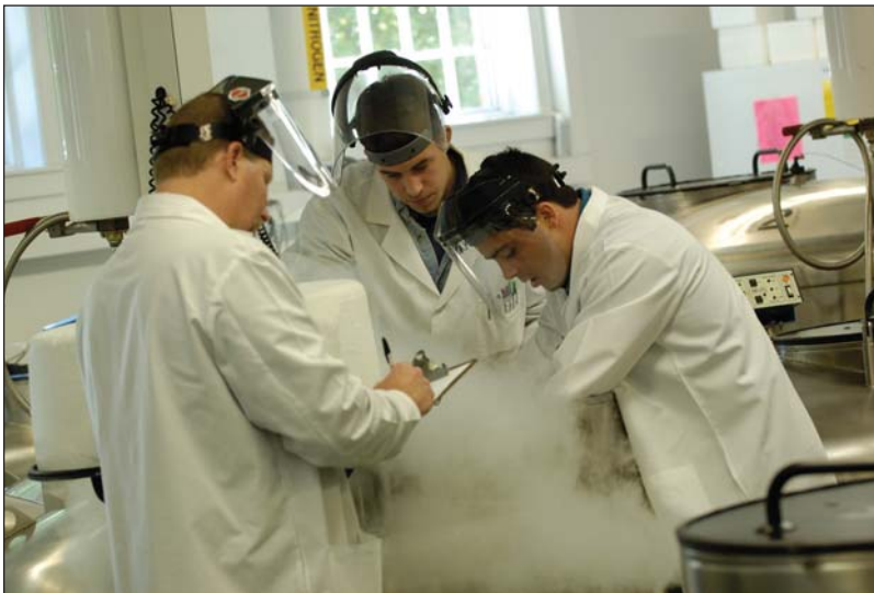
Coriell's cryogenic technicians working in a tank within the Coriell BioBank. Each tank holds 36,720 vials of cells or DNAs, which are distributed around the world for scientific research.
